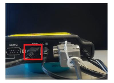
• Make sure that the DC IN cable is connected and that the AC adapter is plugged into a working electrical outlet.
