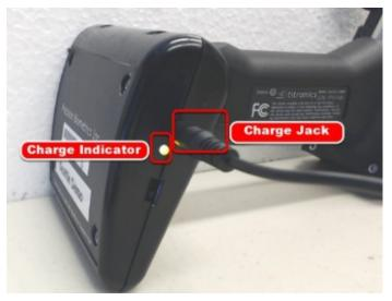
3. Most devices will take 4 hours to fully charge. Once the charge indicator turns green, the device is fully charged and ready for use.
