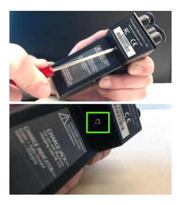
Unscrew it from the device and pull the front end piece off. You may need to give a gently wiggle to loosen. Make sure to keep the screw as you will need it to screw the new front end back to the base piece.
