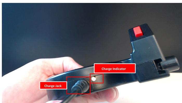
To charge using the wall plug; plug the USB end into the wall charger and connect the wall charger to a power outlet. When the device detects power, the "Charge Indicator" will turn amber. The "Charge Indicator" will turn green when the charge cycle is complete.
