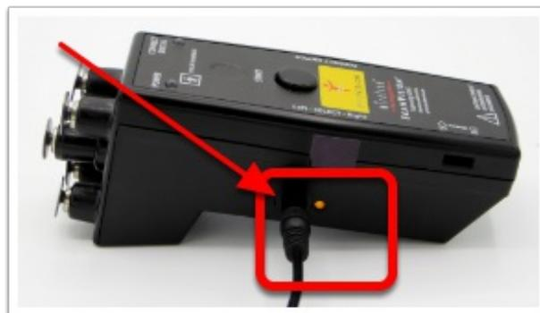
While charging, ensure the charging cable has enough room and is not being bent. If the charge cable is bent while charging, it can cause the charge jack to become loose and potentially cause the charge jack to malfunction. Over time, the charge cable will wear out. You can replace your charging cable by visiting the [MyoVision Store](#) .
