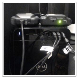
If your computer doesn't have enough USB ports you can purchase a USB hub. A USB hub allows you to convert one USB port into several USB ports.
