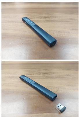
• After plugging the USB Bluetooth adapter into the computer, make sure that the Wireless Remote is powered on. The On/Off switch can be found on the left side of the remote.
