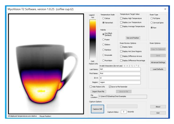
• We can see how the heat is concentrated towards the bottom of the coffee cup because it is only half full. Notice, also, how the heat radiates from the hot water and how the temperature is cooler towards the edges.
